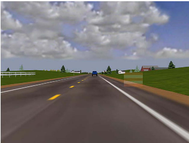
Fig. 2. A view of the driving monitoring task in the simulator. In this case, the image is at the 'near' position and the large size on the right-hand side of the driving scene. The image was chosen to resemble a construction barrier type of barrel.
